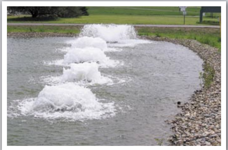
Surface aerators were designed first for the fish farming industry. They can also be used to aerate shallow recreational ponds.
