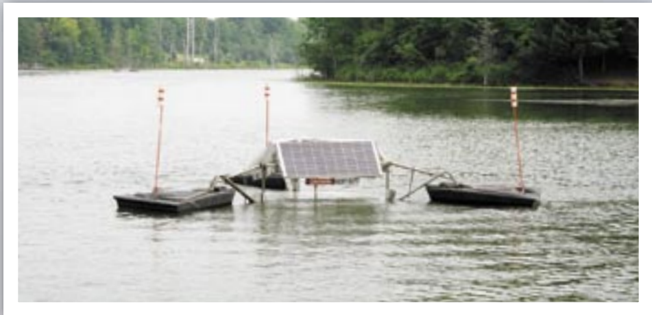
A deployed unit, doing what it does, lifting water from the depths and moving it upward and outward.
