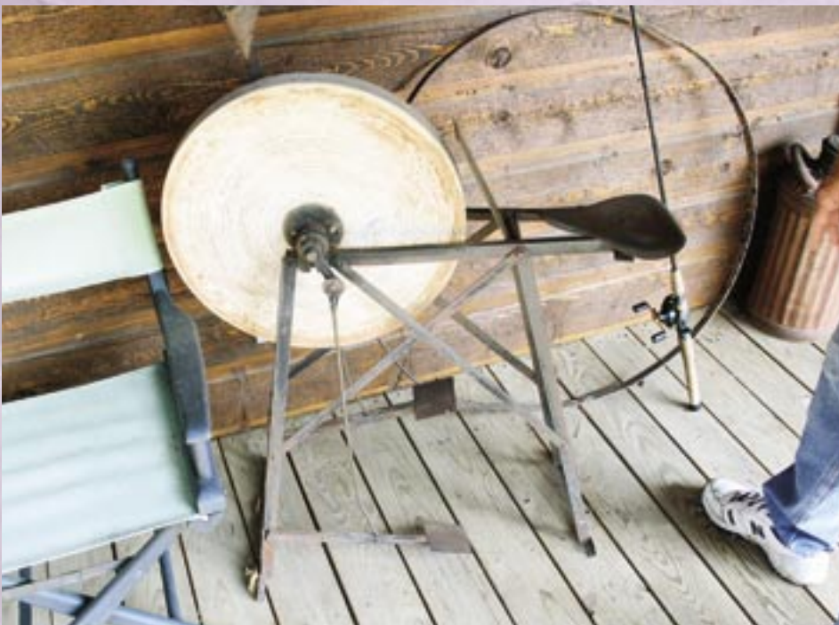
This foot powered sharpener sits on Martin's porch. To this day, he still uses it to keep yard and garden tools sharp and ready.
