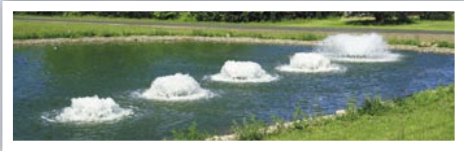
These machines are designed to aerate shallow ponds, primarily for fish hatcheries. Photos for this story compliments of Kasco Marine, Inc.
