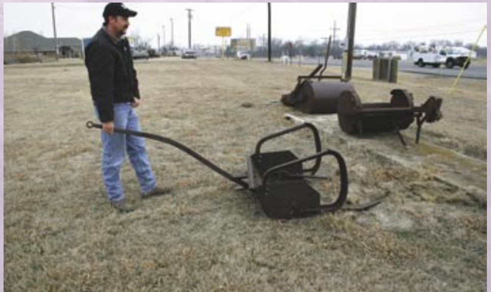
This is a "slip," also called a "Fresno." Pulled by a mule and managed by a human, it was a slow, but effective way to move dirt, way back when.
