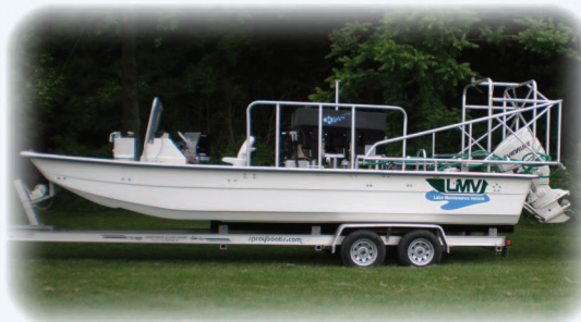
Wet Granular Eductor System on a 25 ft. platform
